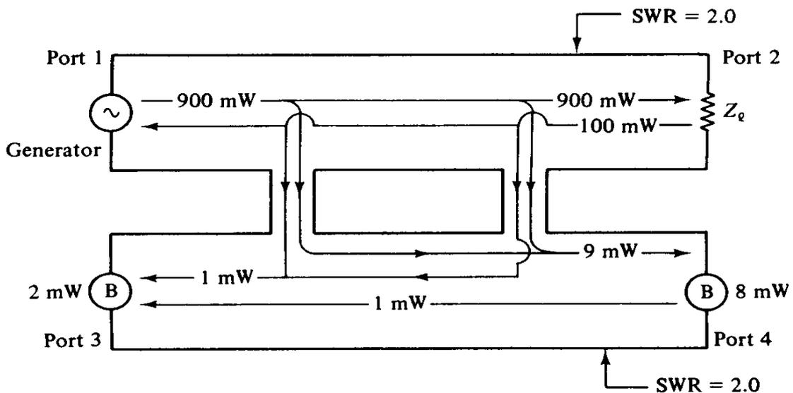
Figure 4-5-5 Wave propagation in the directional coupler.
