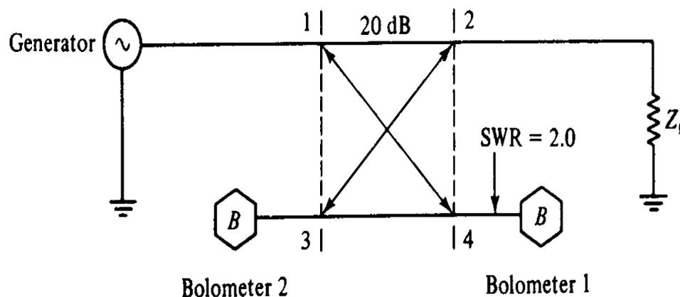
Figure 4-5-4 Power measurements by directional coupler.
