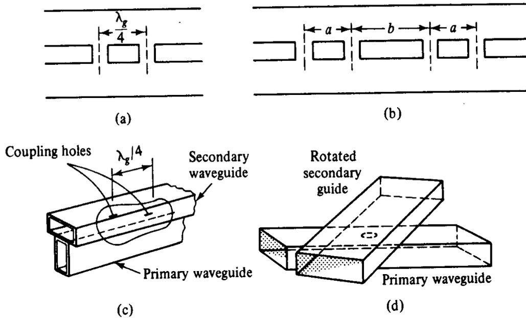
**Figure 4-5-2** Different directional couplers. (a) Two-hole directional coupler. (b) Four-hole directional coupler. (c) Schwinger coupler. (d) Bethe-hole directional coupler.
