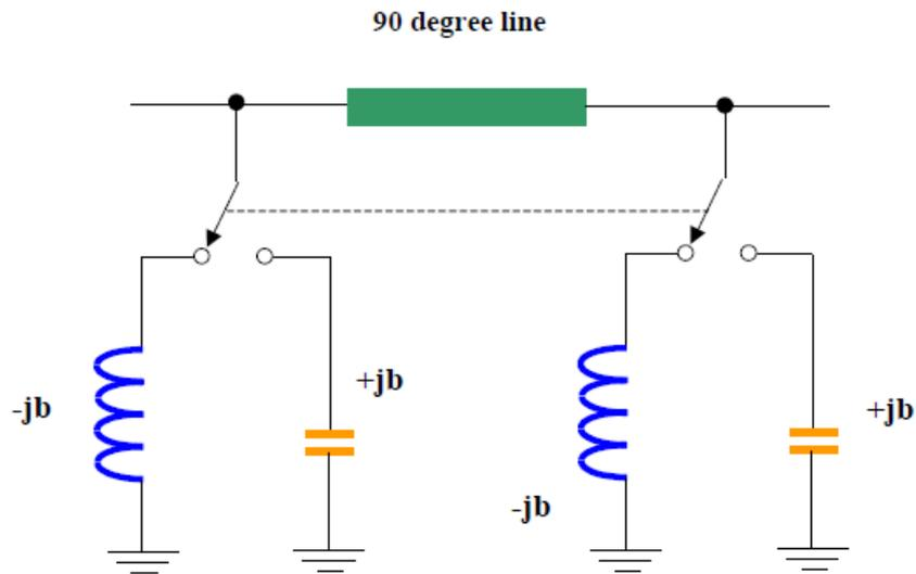
Figure 3 Improved switched-line phase shifter using two shunt susceptances and a quarter-wave length of transmission line.
