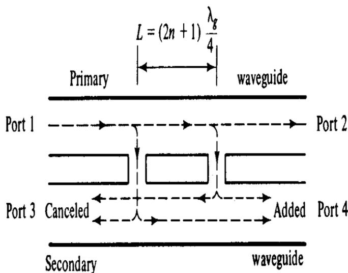
**Figure 4-5-3** Two-hole directional coupler.
